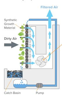
Filtered air is drawn into the building's air circulation system or circulated using onboard fans.
